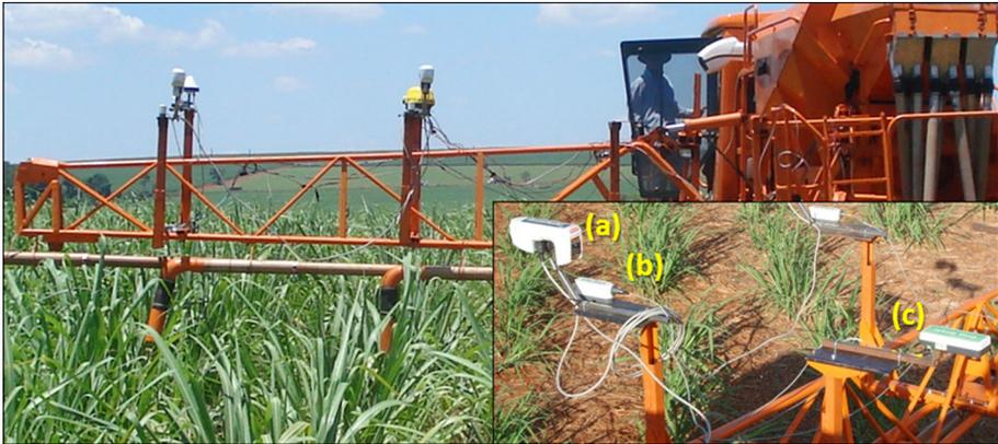
**Fig. 1** The (a) GreenSeeker, (b) Crop Circle ACS-210, and (c) Crop Circle ACS-430 canopy sensors mounted on the fertilizer application boom of a high-clearance vehicle
